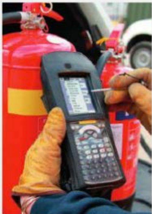
RFID tags can store data relating to health and safety inspections
