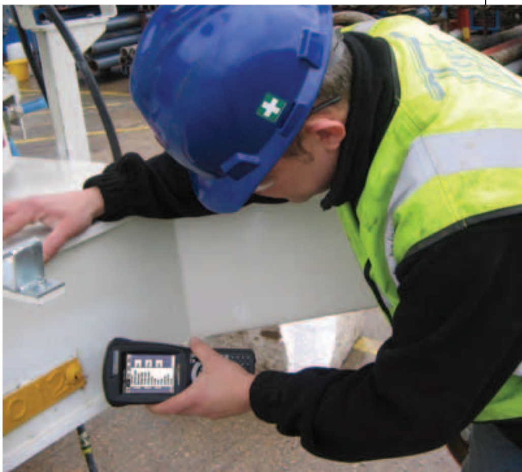
Scanning of an encased tag on a crane.
